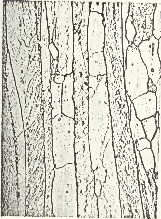
FIG. 23 AT 540°C, UNDER .6%/HR. STRAIN RATE, FOR 18 MINUTES (ROCKWELL 30T 58.9)
